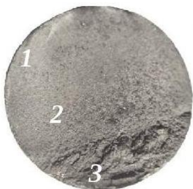
Fig. 8. Fatigue failure with characteristic zones
