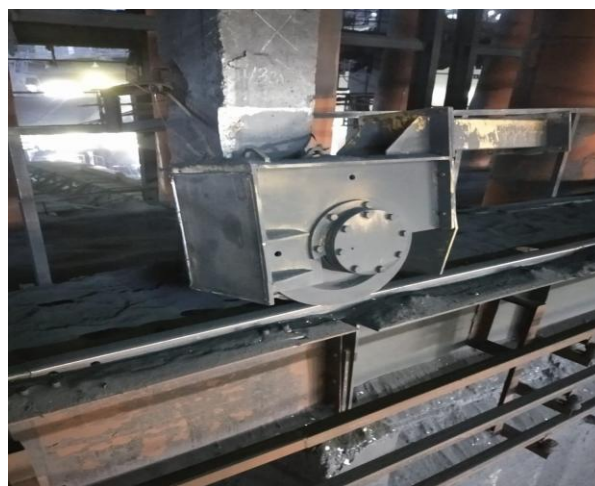
Fig. 3. Complete destruction of welded joints along the metal boundary of the fusion of the walls of the free wheel module with the vertical sheet of the end beam from the side of the trolleys
