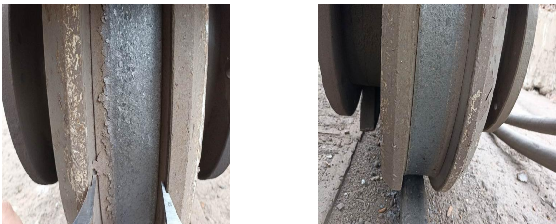
Fig. 5 Wear of the working surfaces of the running wheels
