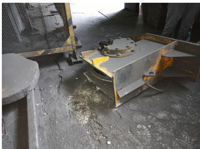
Fig. 2. Complete destruction of welded joints along the metal boundary of the fusion of the walls of the free wheel module with the vertical sheet of the end beam from the side of the crane operator's cabin
