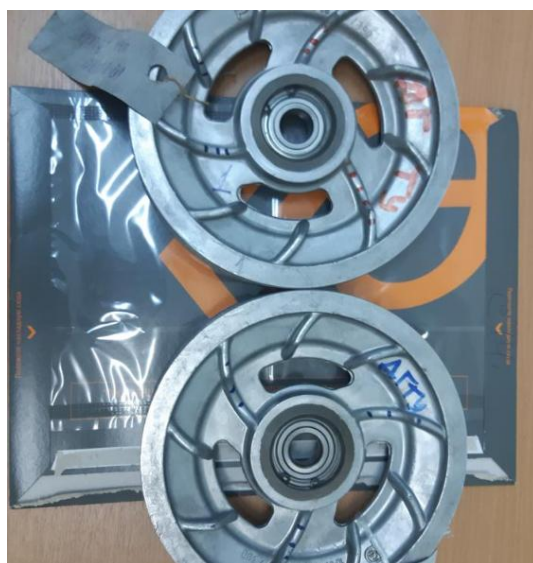
Fig. 1. Belt pulleys of the TORUM 750 combine harvester of the Rostselmash company
