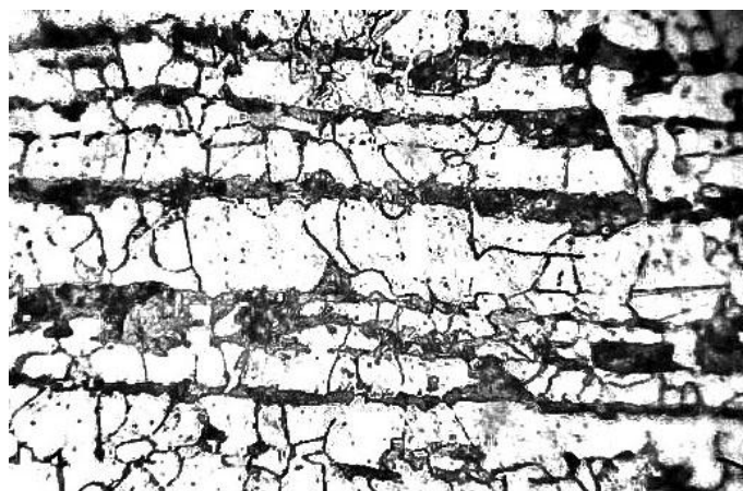
Fig. 2. 14G2 steel with NPMC structure after quenching from 780 °C (29 % martensite), \times 360
