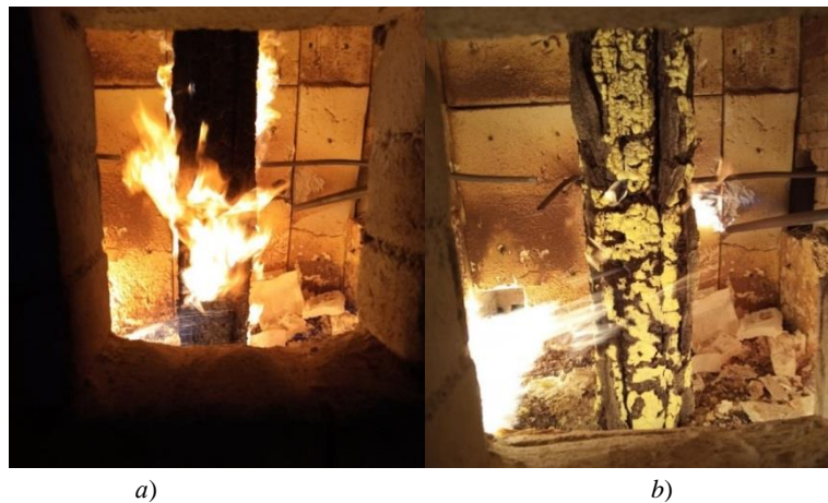
Fig. 1. Fire test result in a standard furnace of I-beam column with an intumescent coating of composition 1: a — 10 minutes after the start of firing; b — after 30 minutes
