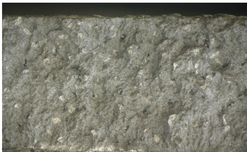
Fig. 1. The appearance of the fracture of melts 5–8 (magnification \times 6.5 )
