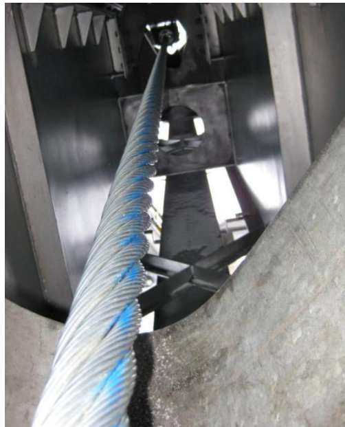
Fig. 5. Control line of axial displacement (torsion) of steel rope around its axis
