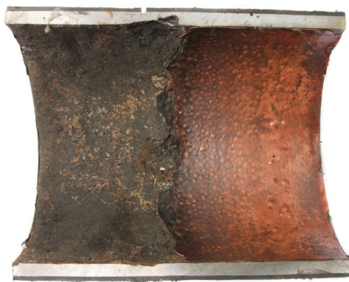
Fig. 5. Destruction of the internal anticorrosive coating of the pipeline \text{Ø}159 \times 8 mm
