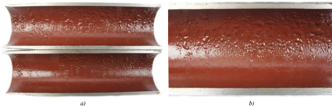
Fig. 1. Damage to the internal anticorrosive coating: a, b — coating blistering
