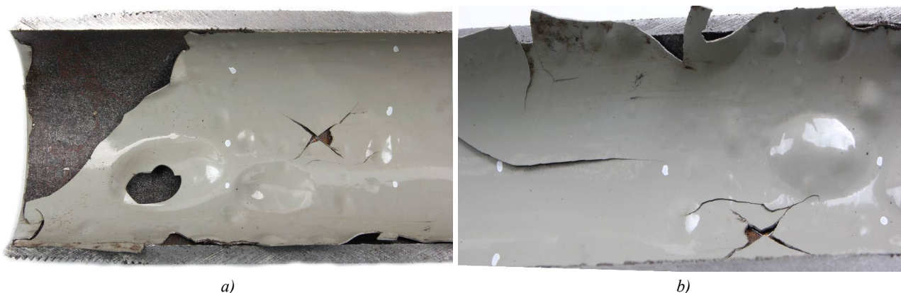
Fig. 2. Destruction of the internal anticorrosive polymer coating: a — blistering of the coating; b — cracking of the coating
