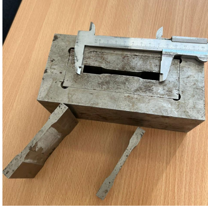
Fig 5. Laboratory mold for the manufacture of tensile test samples according to GOST 8227-98 for cold-pressed and sintered samples
