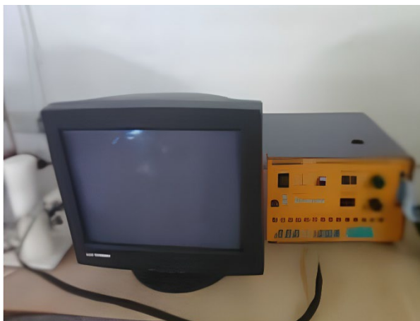
Fig. 2. Device for determining the coefficient of thermal conductivity
