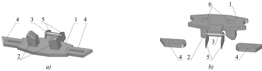
Fig. 4. 31883-NSB folding double welded stop [12]:
