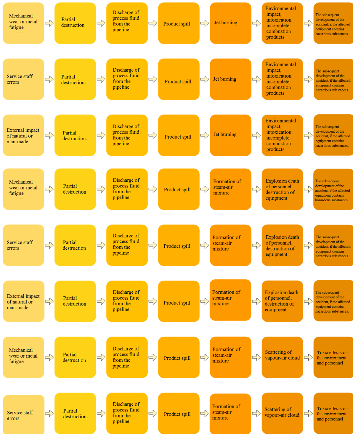
Fig. 3. Scenarios for the development of an emergency situation with the complete destruction of the process pipeline
