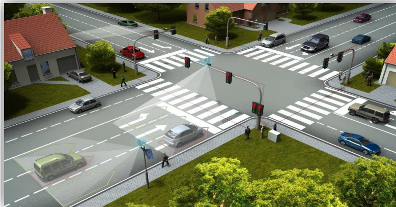
Fig. 5. Layout of sensors at a conditional intersection
