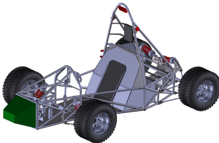
Fig. 2. Design of a racing car designed according to the FSAE regulations, with an energy-absorbing element (indicated in green)
