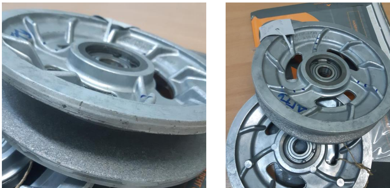
Fig. 3. Belt pulleys after nickel alloy spraying
