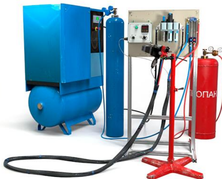
Fig. 2. Installation for gas-thermal surfacing of the Rostselmash company
