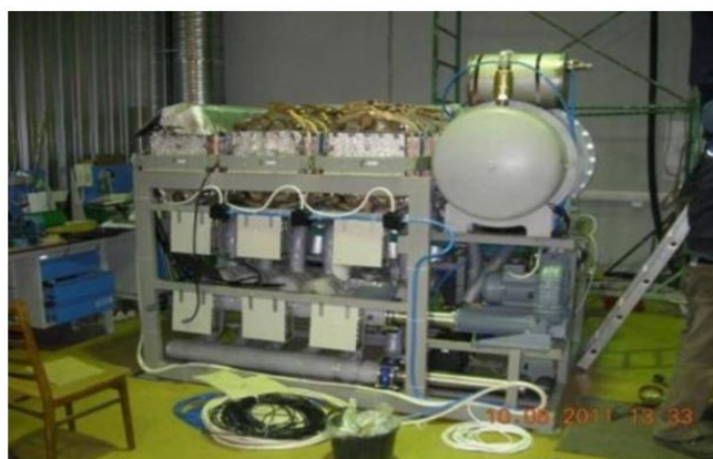
Fig. 8. Marine hybrid power station based on BTE-84 batteries with a capacity of 60 kW/ [10]
