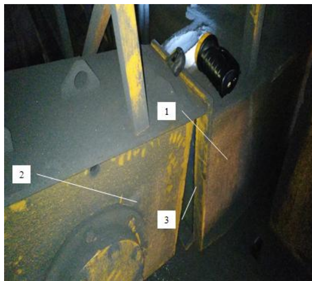
Fig. 5. Modular design of the end beam with a welded flange connection (photo by the authors): 1 — metal structure of the end beam; 2 — running wheel module; 3 — destroyed welded flange connection
