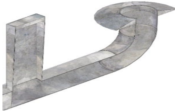
Fig. 5. Cross section of the lower inlet pipe of the secondary dust and gas flow of the CSF dust collector
