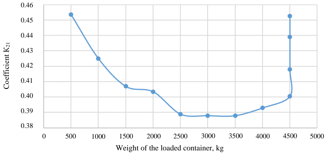
Fig. 5. Dependence of K_{21} coefficient on the weight of the loaded container with a cable car with a length of 20 thousand meters
