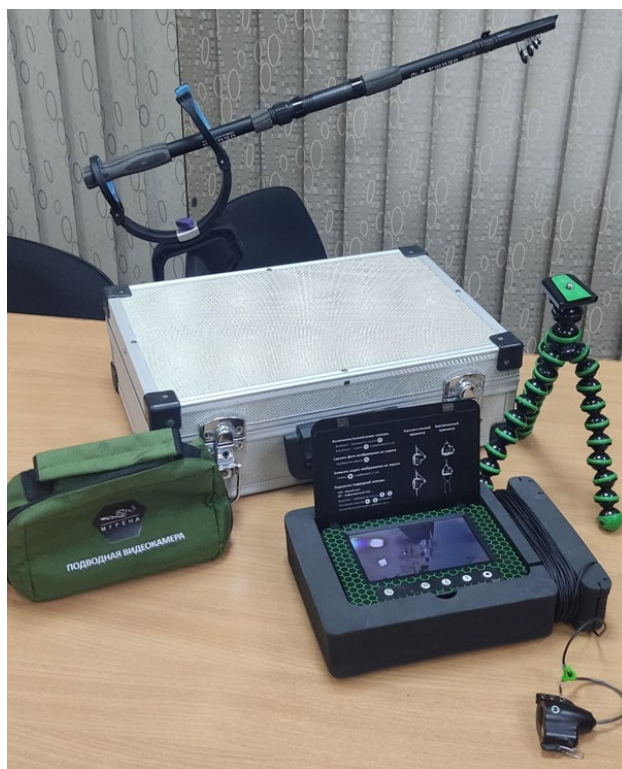
Fig. 3. The case and the surface unit of the Praktik Murena video camera
