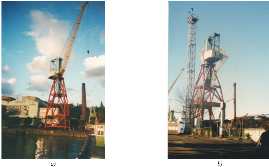
Fig. 3. An accident of a portal jib crane due to the destruction of the lifting mechanism: a — before the accident; b — after the accident
