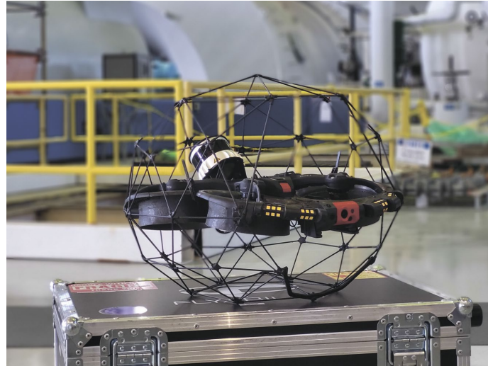
Fig. 1. Industrial inspection FPV drone (quadcopter) with protective frame
