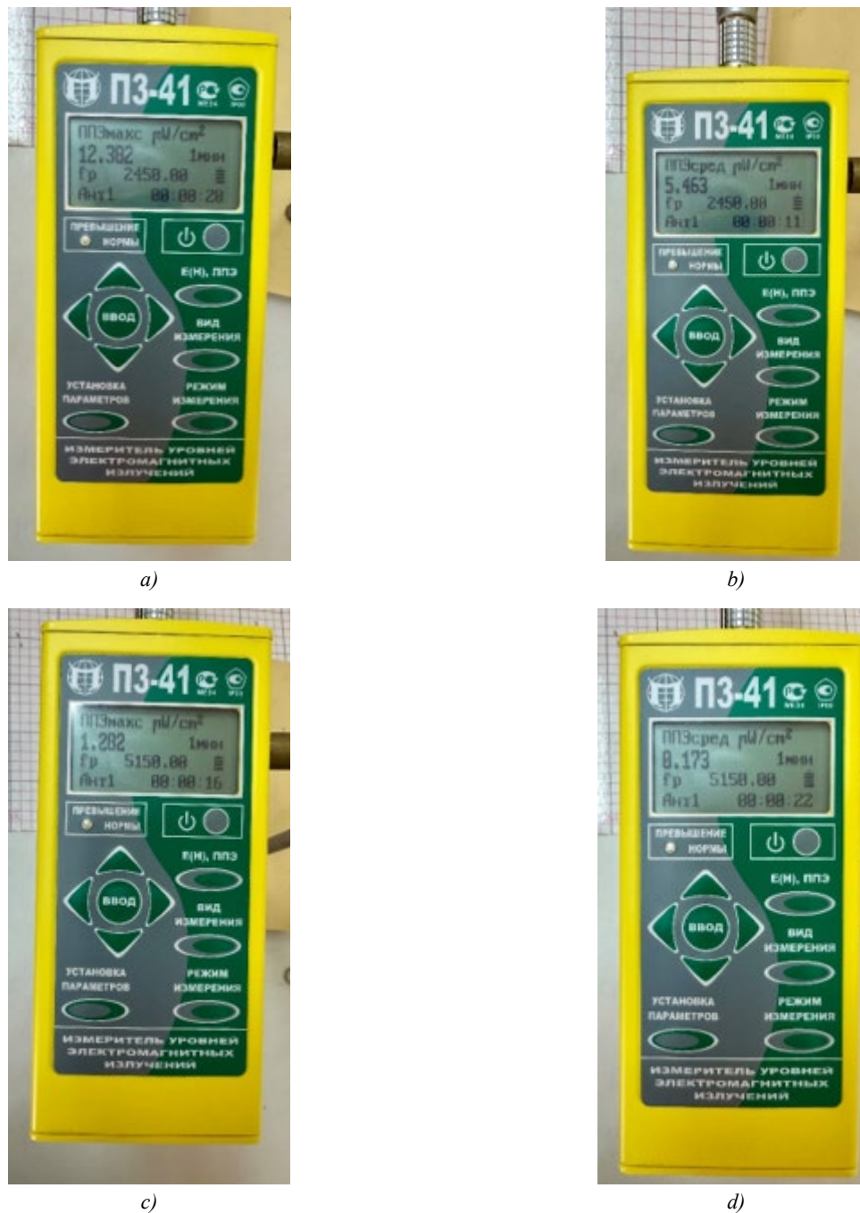
Fig. 1. PZ-41 device interface when measuring EFD max and EFD avg at frequencies of 2450 MHz and 5150 MHz a — determination of EFD max at a frequency of 2450 MHz; b — determination of EFD avg at a frequency of 2450 MHz; c — determination of EFD max at a frequency of 5150 MHz; d — determination of EFD avg at a frequency of 5150 MHz
